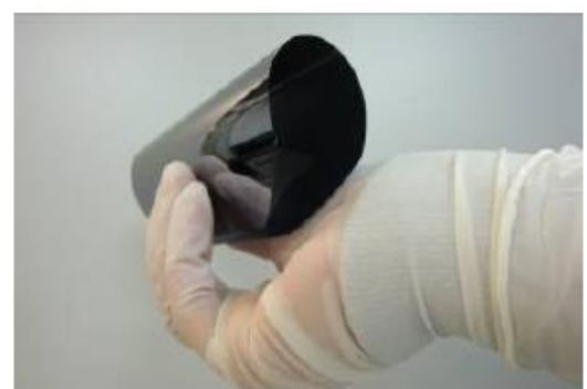
125mm x 125mm – First ever kerf-free 20 \mu m Mono c-Si Solar PV Foil
